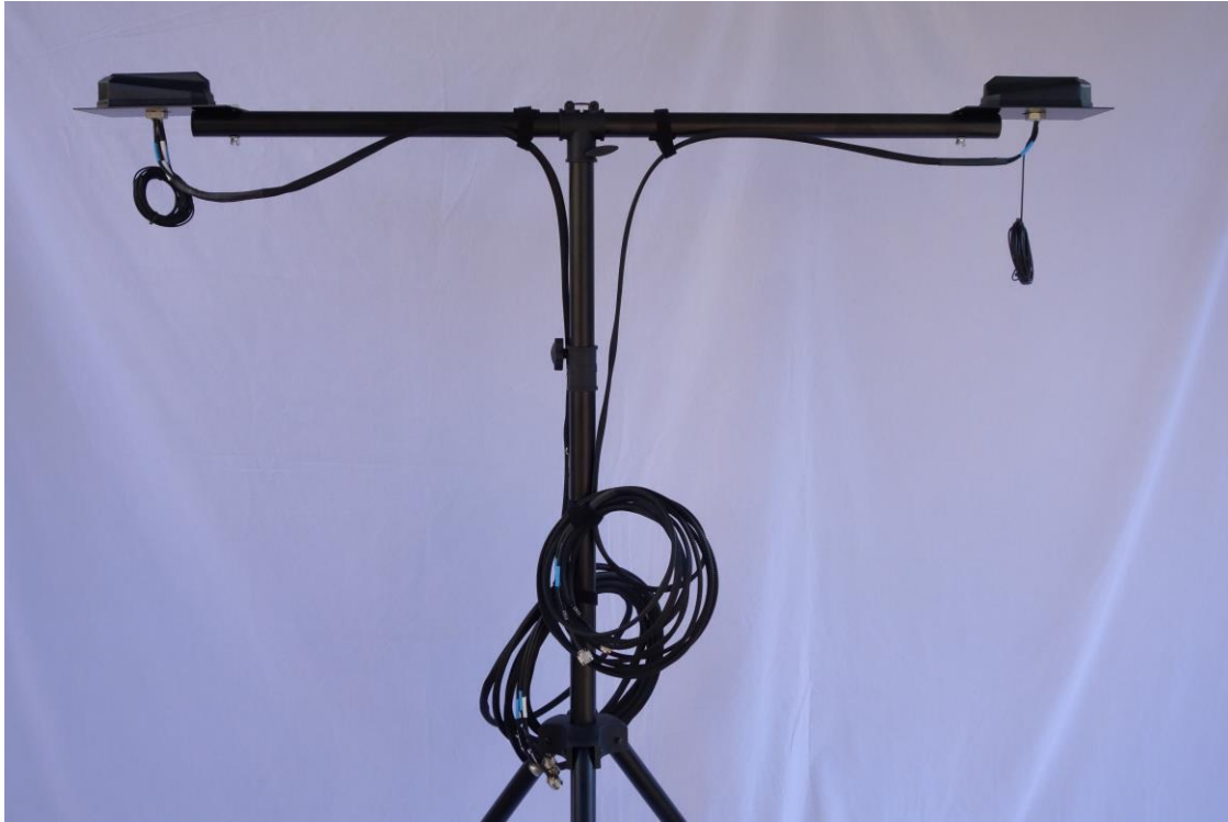
Portable Antenna System with Tri-Pod, cabling, multi-band antennas and connectors
